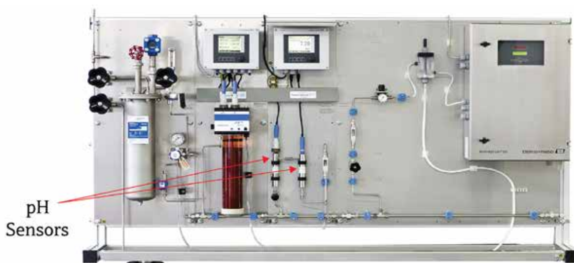
FIGURE 5 pH sensor installation in pre-fabricated panel.
