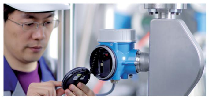
The verification procedure is typically performed within minutes and can be initiated through the display, FieldCare or webserver (if incorporated).
