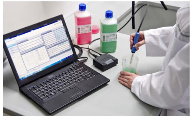
Calibrate your sensors with Memobase Plus in the controllable and comfortable environment of your laboratory.
